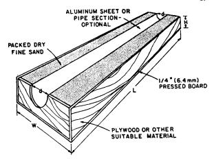
*L* = variable length to suit the length of sampling tube W = d + 2 in. (51 mm) H = d + 0.25 in. (6.4 mm) *d* = outside diameter of sampling tube used
