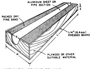
L = variable length to suit the length of the sample d = inside diameter of sampling tube used W = d + 2 in. (51 mm) H = d + 0.25 in. (6.4 mm)
